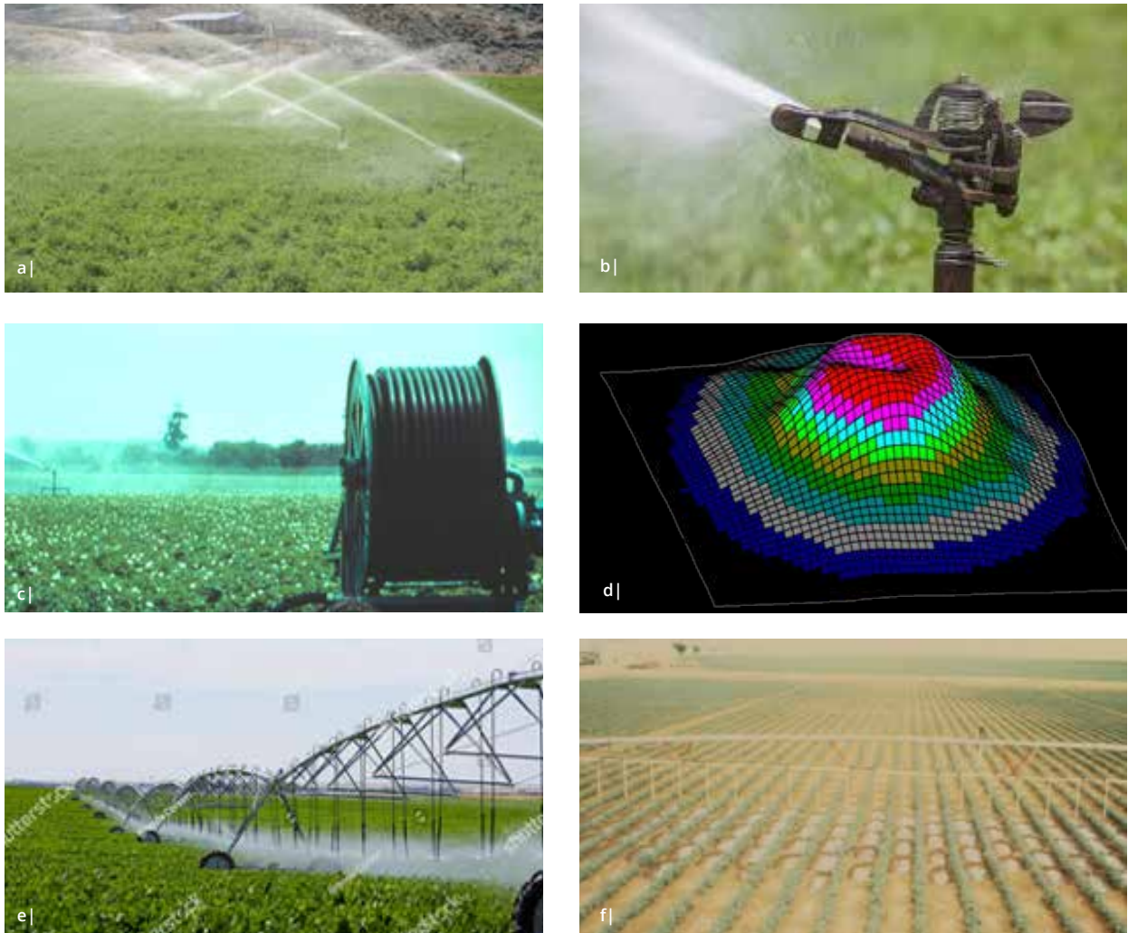
Figure 24 Typical sprinkler irrigation systems a) small rotary sprinkler b) close up of sprinkler head c) mobile raingun d) wetting pattern from a rotary sprinkler e) low pressure centre pivot machine f) putting water where it is needed
