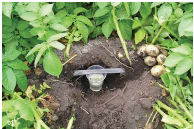
Figure 28 Measuring flow rate from emitters along a drip line a) surface line on grape vines b) buried line on potatoes
