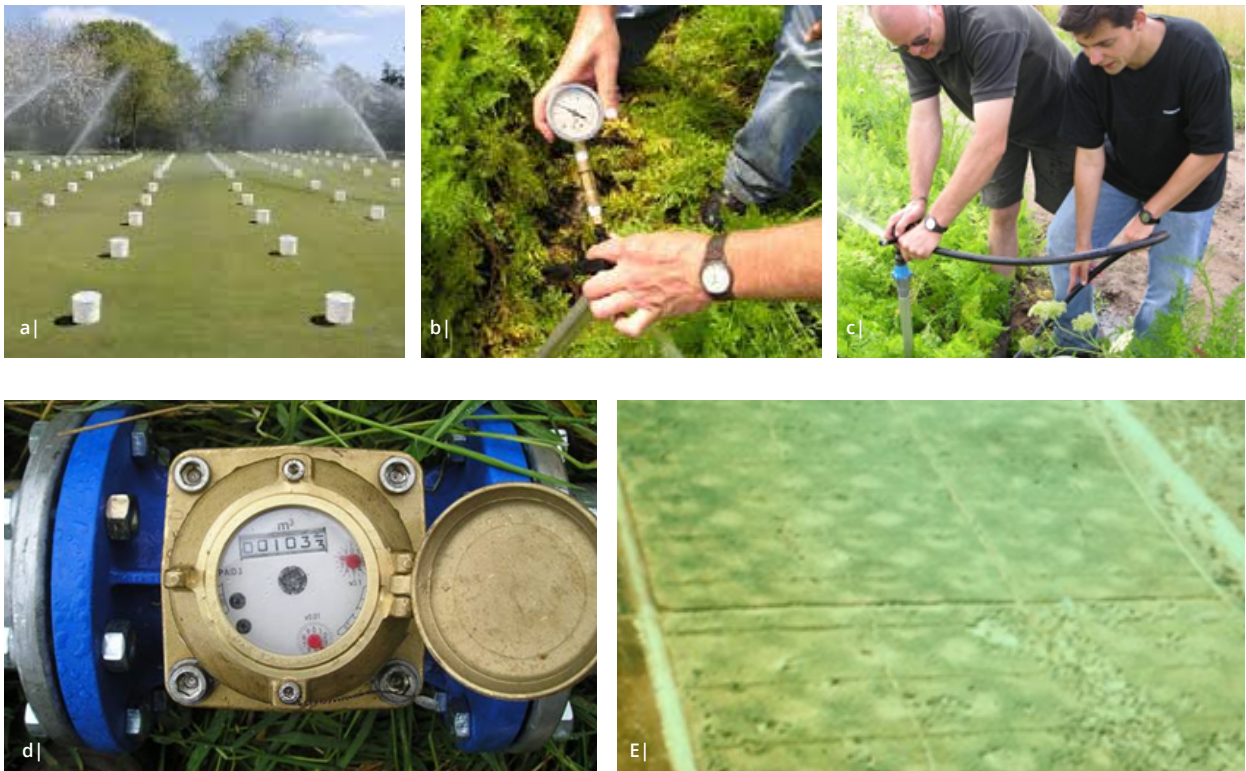
Figure 26 Sprinkler evaluation a) measuring uniformity b) pressure c) discharge from a sprinkler d) flow meter on mainline e) doughnut ring effect in crop when pressure is too low
