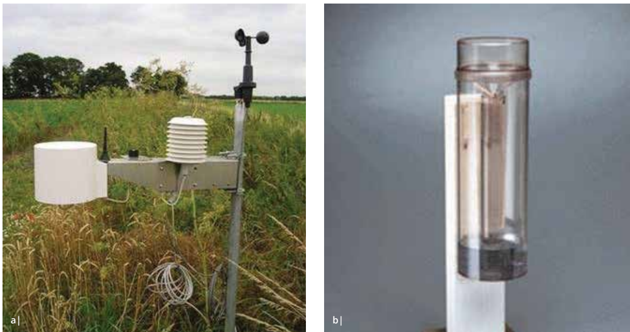
Figure 30 Tools for irrigation scheduling a) automatic weather station b) rain gauge
