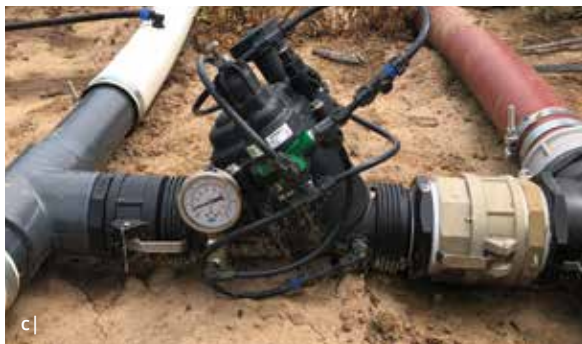
Figure 27 Drip irrigation a) on field scale crops b) drip on protected fruit crop c) pressure control equipment
