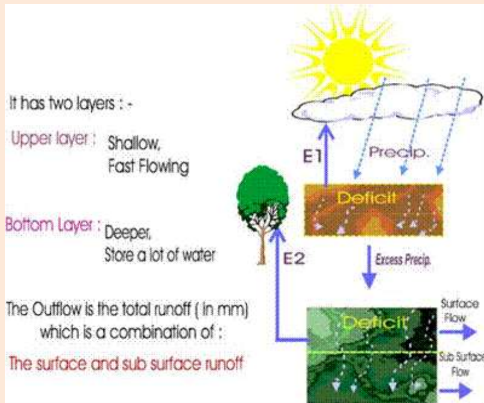
Figure A.II.8. Main Concept of Water Balance Model
