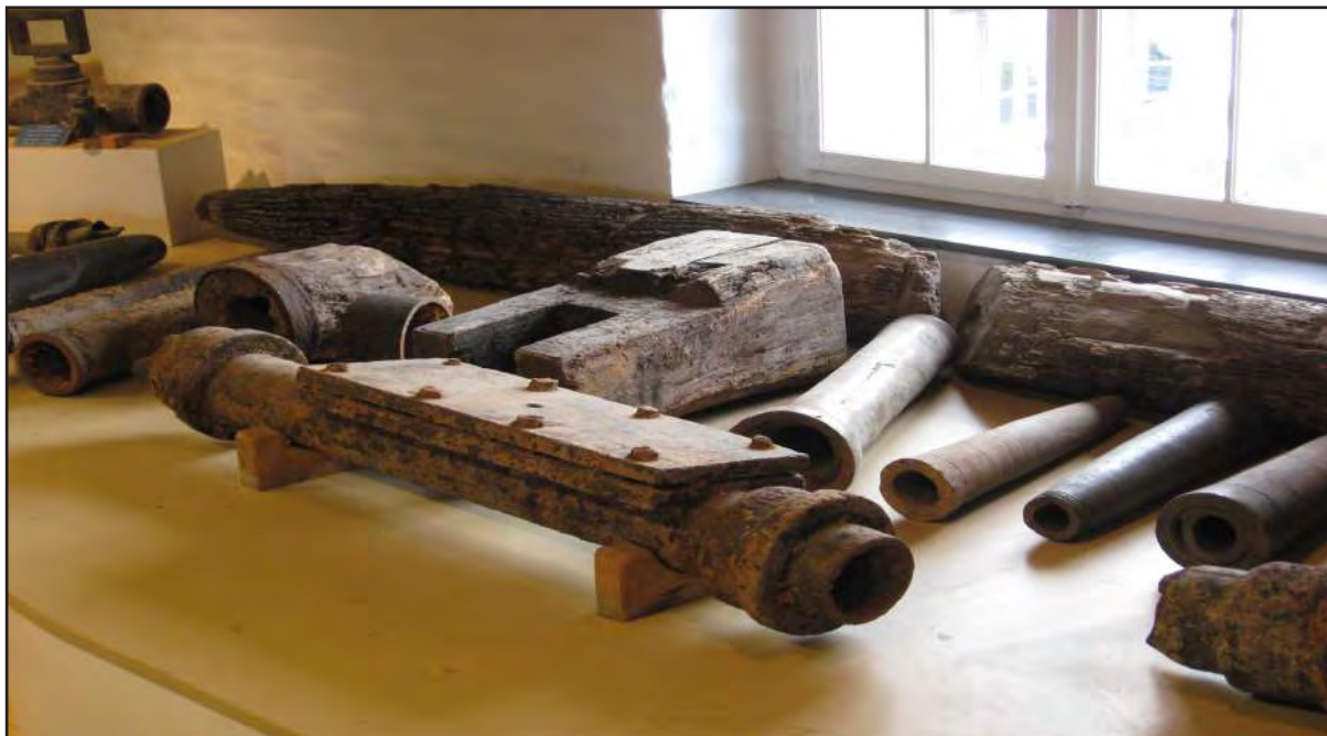
Figure 8. Development of the pipe in the water supply from wooden pipes (rear) to clay pipes (centre) to cast iron pipes (front) (TechniKmuseum Neue Mühle, Kassel)
