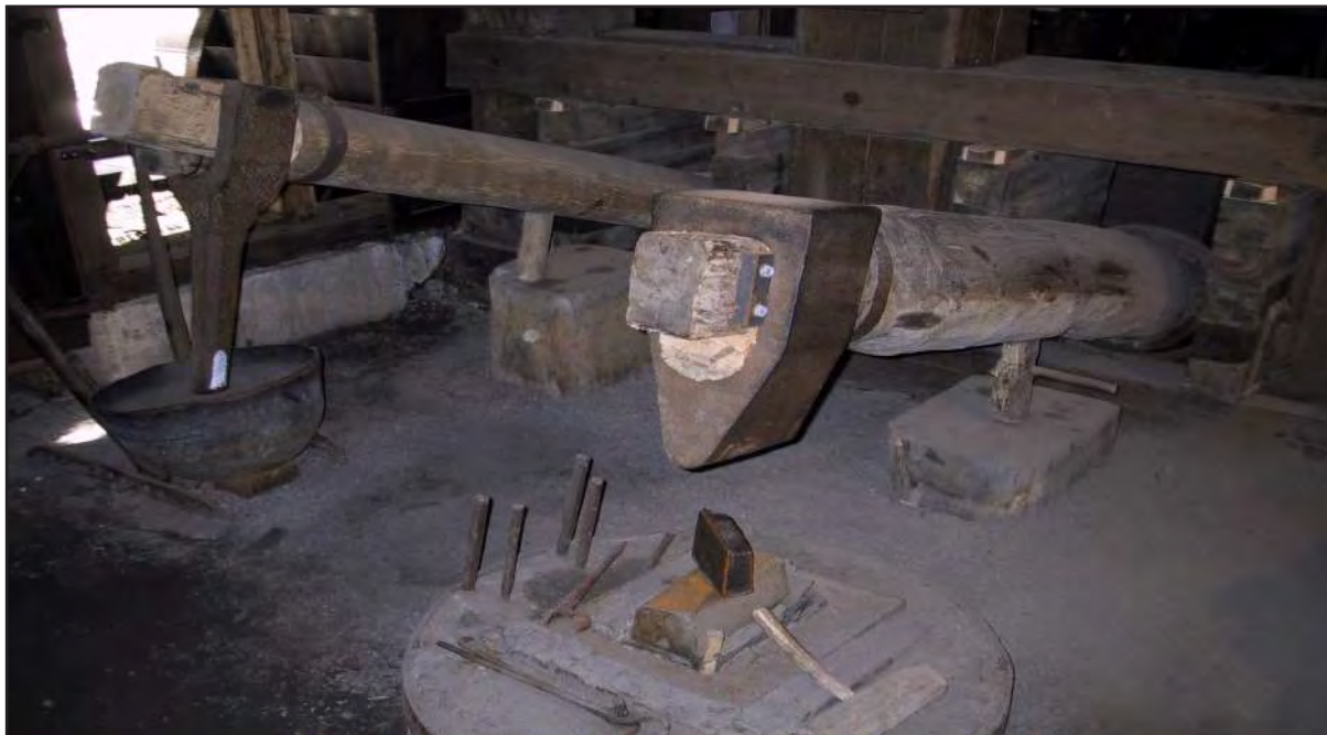
Figure 6. Forging hammer driven by a water wheel (Tobiashammer, Ohrdruf)
