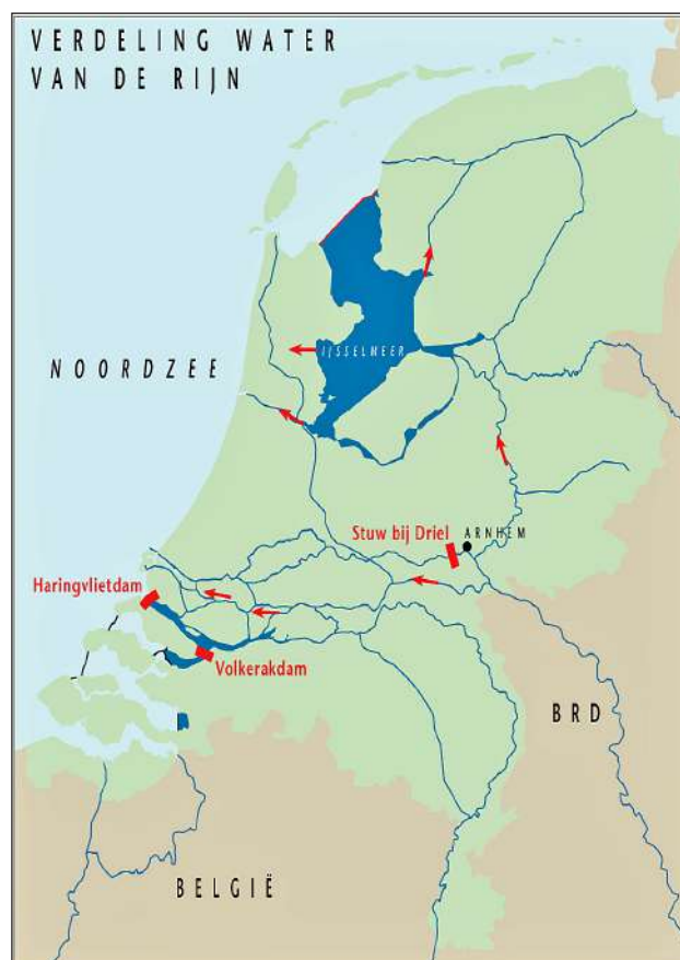
Figure 8. The national hydraulic system, with the weir at Driel a controlled division of water of River Rhine between the branches IJssel and Neder-Rhine has been established, thus ensuring sufficient flow into the IJsselmeer
