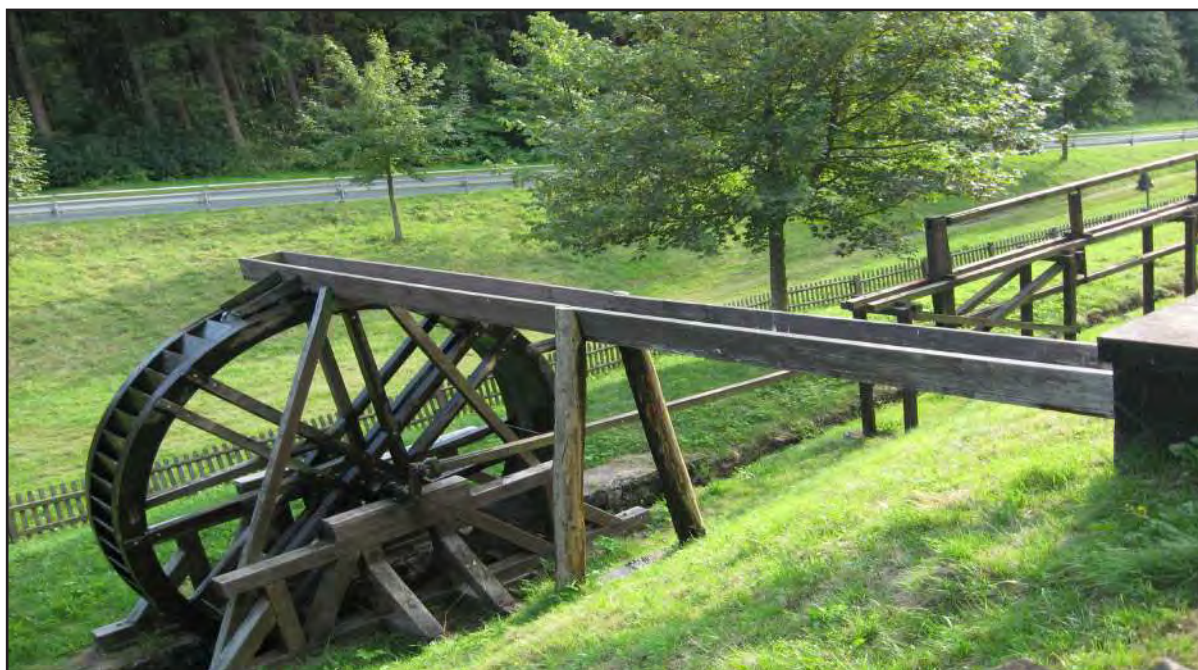
Figure 7. Waterwheel with artificial linkage for transmitting power to the pump (model demonstration, Upper Harz Water Regale)
