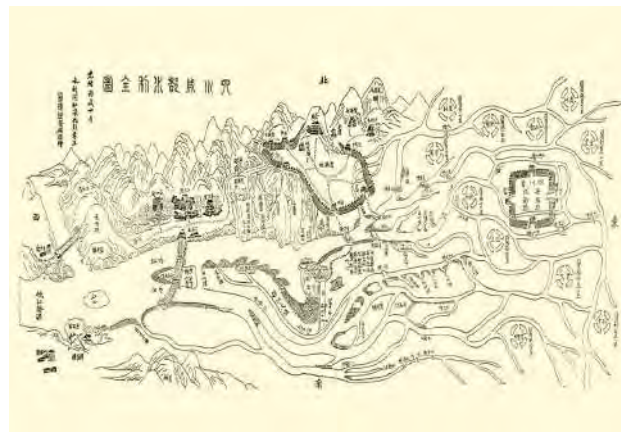
Figure 6. Dujiangyan and the canals on Chengdu Plain (drawn in 1886). Since the 2 nd century Dujiangyan irrigation system has been distributed in the plain.
